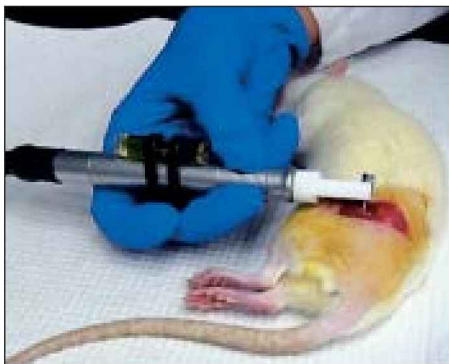
Fig 1 The approach position of the percussion probe to the testing abutment. The supporting arm is not in contact with the animal's head.
